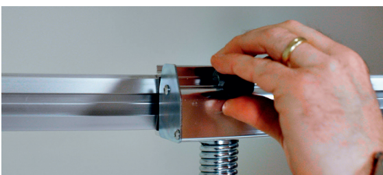
6 Fasten the profiles with the screw.
